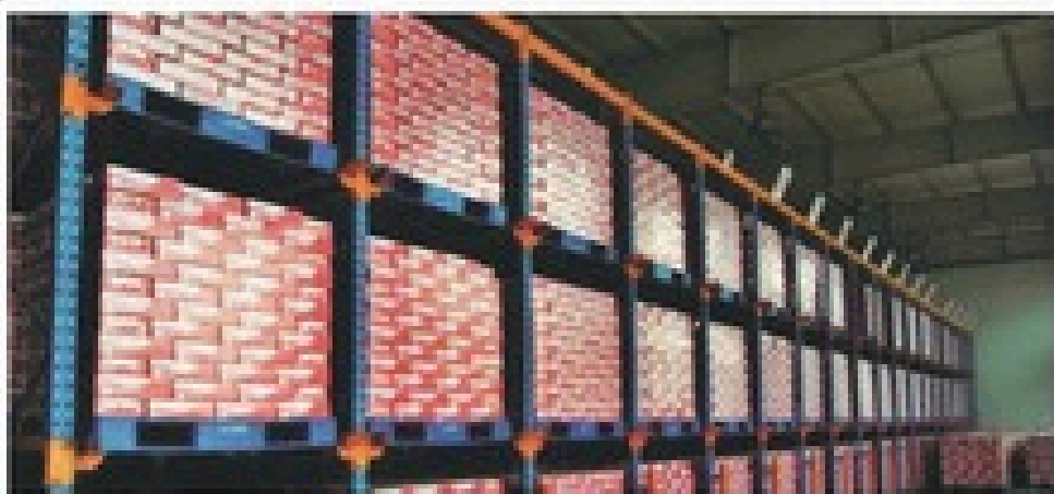
DRIVE-IN RACKING LOAD
